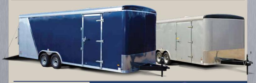
SUPER LOCK... Interlocking Exterior Aluminum system -unique to Haulin Trailers, lasts longer, looks much better, won't rust. The .030 interlocking aluminum panels are glued and mechanically fastened with fewer exposed screws.
